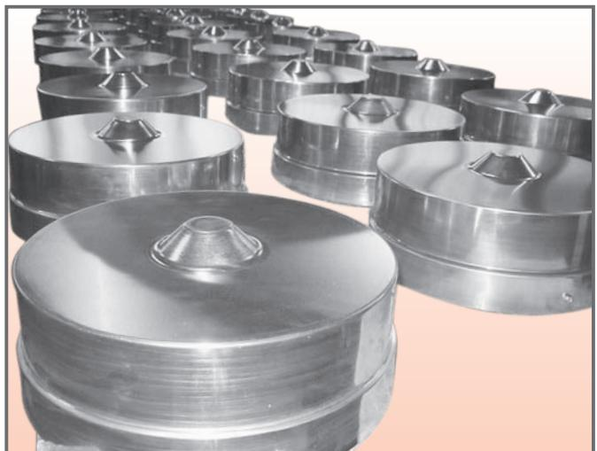
Parts in contact with the product in galvanised mild steel with cover in aluminium
